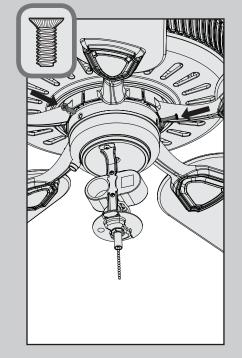
Insert three (3) switch housing screws, found in the  $\equiv$  hardware bag.
